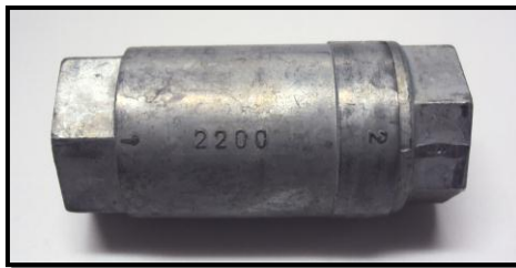
#170148 Sealco 2200/8 check valve 1/2" (female ports both ends)
